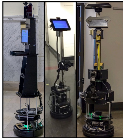
Figure 7: Prototype service robots designed as variations on our low-cost platform, developed by students in CIS 700 at the Univ. of Pennsylvania in Fall 2015. The middle and right robot also include a belt-driven elevator mechanism to raise the manipulator along the mast, using a coil spring to offset the arm’s weight. These robots were used for a variety of tasks, including waiting tables at a simulated restaurant, object search and retrieval, and voice-based navigation.
