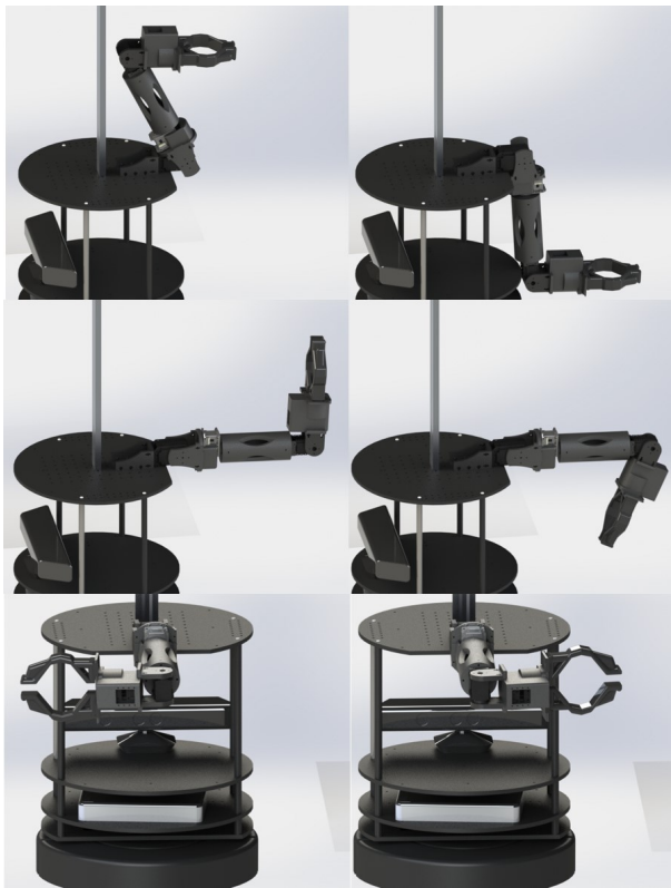
Figure 4: Mobility of the robotic arm.
